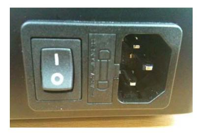
AC input:  $100^240 \text{ V}$ ; 50/60 Hz power source
