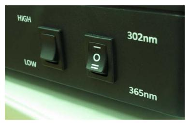
High/Low: Intensity adjustment (100% & 50%) 302/365 nm: Selection of UV lamp wavelength PWR off: central position of the wavelength switch
