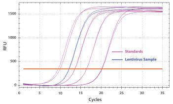
**abm's qPCR Lentivirus Titer Kit enables easy visualization of viral titers.** A lentivirus sample (blue) was processed following the protocol for the qPCR Lentivirus Titer Kit and amplified in a qPCR reaction along with standards included in the kit (purple).
