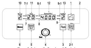
Figure 3: Schematic Drawing of Control
